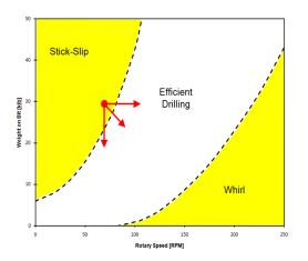
Conventional stick-slip mitigation can produce sub-optimal performance given a smaller efficient drilling window.
