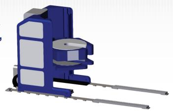
Replacing the need for casing crews and manual tongs, the electric roughneck is capable of handling high torque (250 kNm) and enables full control of all parameters. It can be used for various sizes of both drill pipe and casing. The height of the torque wrench and backup tong can be individually adjusted to handle bottom hole assemblies and other challenging drilling operations
