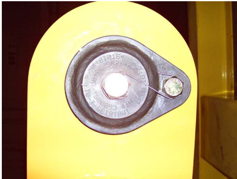
Figure 3 – Bolt with Loctite and Safety Wire installed in Extraction Hole
