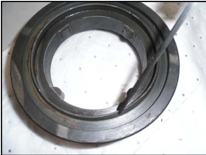
Figure 1: Old spacer design with damaged rib
