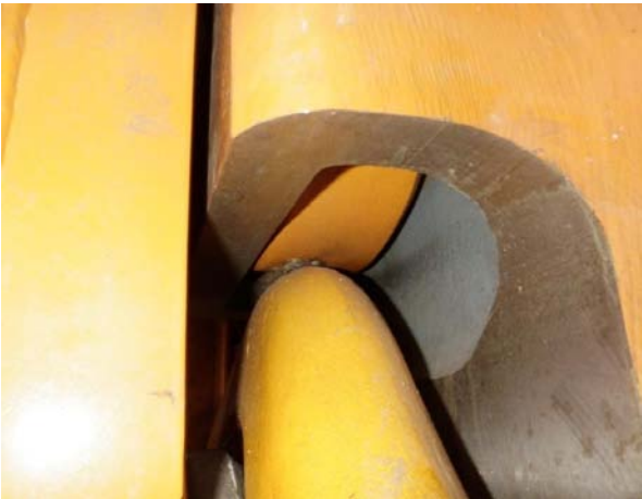
Figure 1: Elevator link in contact with gearbox and split block adapter
