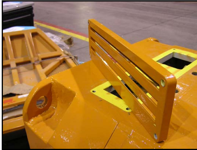
Figure 3: Remove louver to access bolts inside motor main body frame
