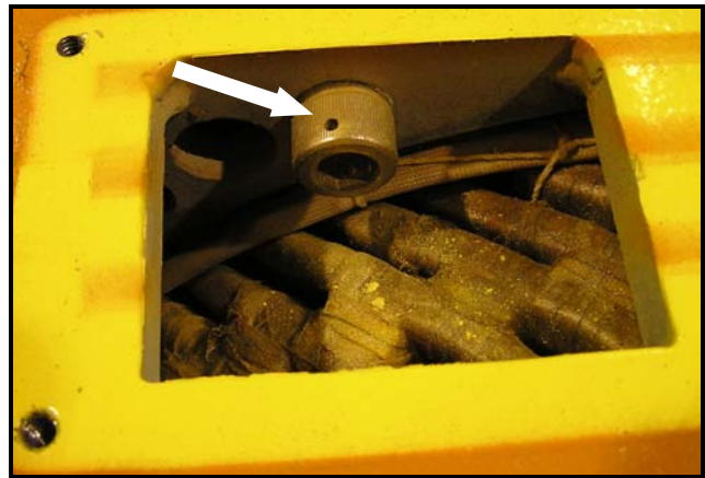
Figure 2: Close-up view of bolt in motor main body frame
