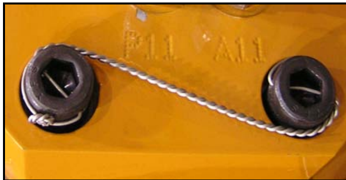
Figure 4: Example of bolts that are properly lock wired
