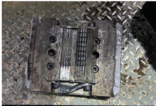
Figure 1: Damaged Grabber Die Holder Plate
