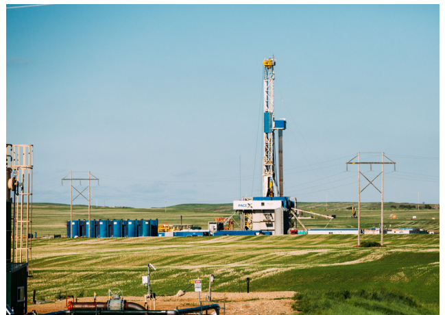
Photo: The PACE®-X Rig is operating in the Bakken region using highline power.
